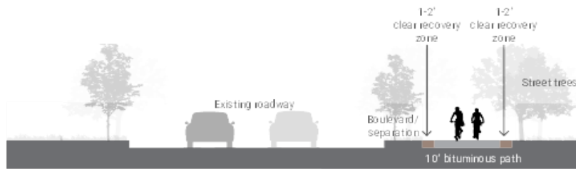
Figure 3-18. Fergus Falls GET: Adjacent to Roadway Typical Section
